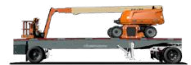
SHIPPING MODE Allows the entire boom lift to be lowered for tie-down and transport, maximizing clearance and maneuverability and allows for transport without costly oversize permits.
