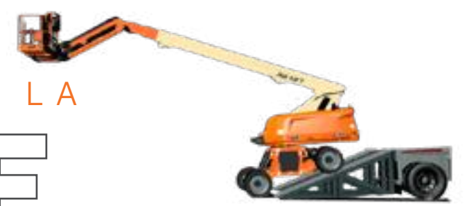
SELF-LEVELING MODE Machine automatically adapts on slopes up to 10 Degrees.
